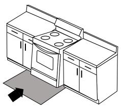
C. Standing on top of Masonite-Hardboard / Scuff Shield pull appliance onto the Masonite-Hardboard / Scuff Shield. Do not slide Loaded sheet across the Floor with appliance on top.
