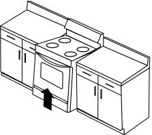
B. Insert edge of Masonite/ hardboard (shiny side down) under the front of the appliance.
